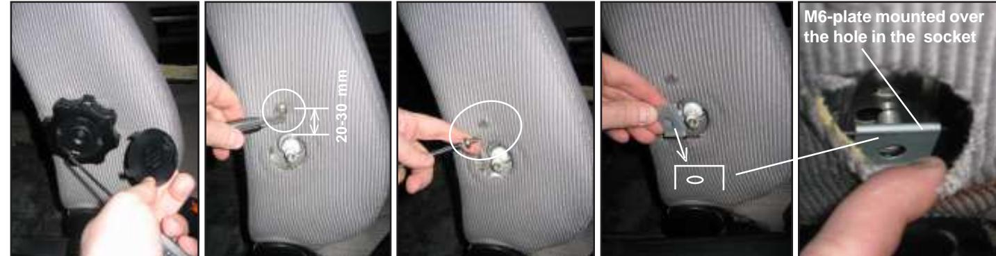
Remove the adjustment wheel/ Cut a hole over the screw-head (appr. 20-30 mm over the adjustm-wheel) and remove the screw. For the lower securement point -Mount the M6-plate over the socket that is placed behind the upholstery. Cut a small hole and centre the M6-plate with the hole in socket, by running a screwdriver from the outside.
