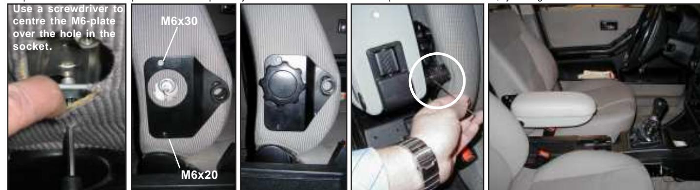
Mount the bracket with the enclosed screws. Restore the adj-wheel before you tighten the screws hard. Mount the armrest and secure it by tighten the lock-screw on the adapter.
