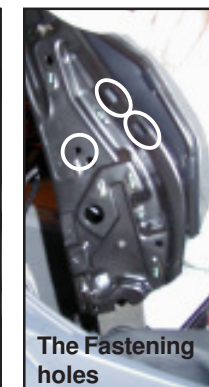
Mount the adapter in the pointed holes.
