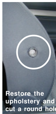
Fold back the foam and cut a hole for the tube.
